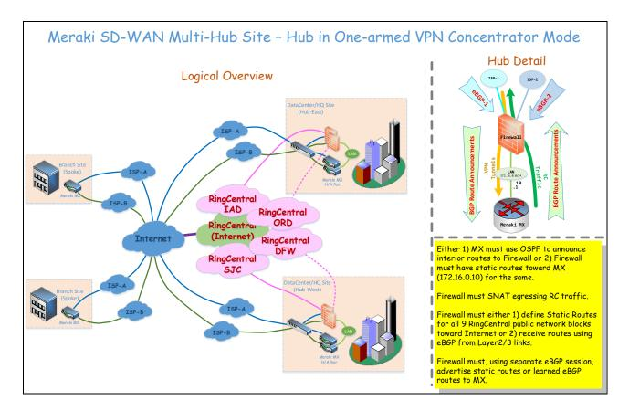
In this mode, the Meraki has only one active port, WAN1, which is connected to and assigned an address as part of the LAN. The LAN is connected to a firewall device which manages the ISP links. The firewall device must provide SNAT services for the RingCentral traffic and 1:1 DNAT/SNAT services for AutoVPN tunnel origination/termination. An iBGP session is established between the Meraki appliance and the firewall device.
