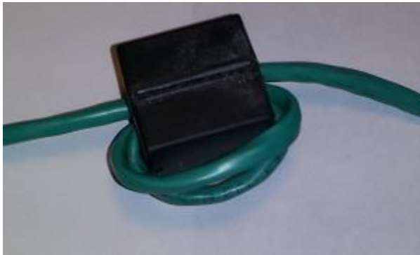
Figure 3 - Clamp-on Ferrite Choke with multiple cable turns. Note that the diameter of the loops pictured is too small. The picture below shows the proper size of the loops.
