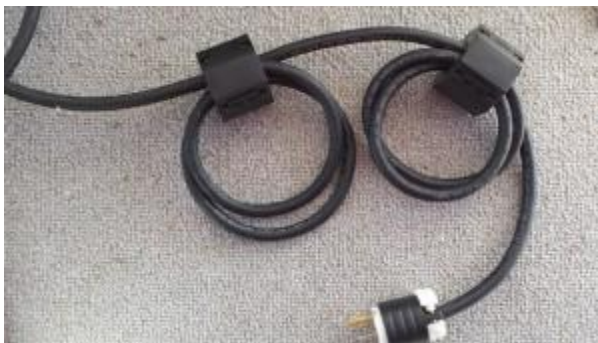
Figure 4 - Use of multiple Ferrite Chokes with multiple cable loops
